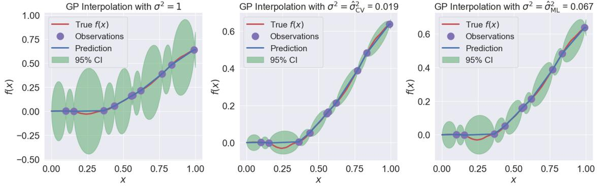
**Figure 2.** GP interpolation of an integrated fractional Brownian motion with the Hurst parameter  $H = 0.5$  (smoothness  $l + \alpha = 1.5$ ) using the Brownian motion kernel (1.2) with three different scale parameters:  $\sigma^2 = 1$  (left),  $\sigma^2 = \hat{\sigma}_{CV}^2 = 0.019$  given by the LOO-CV estimator (middle) and  $\sigma^2 = \hat{\sigma}_{ML}^2 = 0.067$  obtained with the ML estimator (right). For the explanation of the figures, see the caption of Figure 1.
